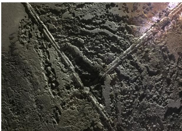
**Figure 2.** Example of severe pitting corrosion of a tank bottom and weld joint (where proper mechanical, operational, and chemical corrosion mitigation procedures were not followed).
