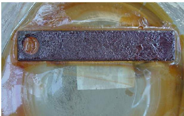
**Figure 3.** Thin film corrosion developed on coupon after loss of ammonia.
