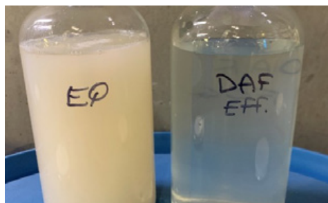
EQ tank water vs DAF effluent water utilizing the new treatment strategy.
